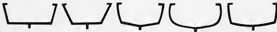
Sailboat hull shapes: Left to right —flat-bottom, modified flat-bottom, V-bottom, round-bottom, and arc-bottom
